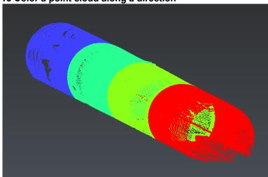
Now we can explode the point cloud according to the colors we have just set. Select the point cloud and got to Inspection Steps. The four sub clouds are added into the Measure Group and you can work on each one separately.
