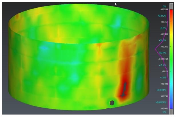
109 Compute the 3D deviations on the tank shell
