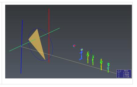
Launch the command <u>Distance</u> <u>between Points</u> and select the middle of the blue line and the middle of the red one.
