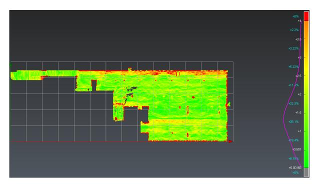
92 Check the slopes on a concrete floor
