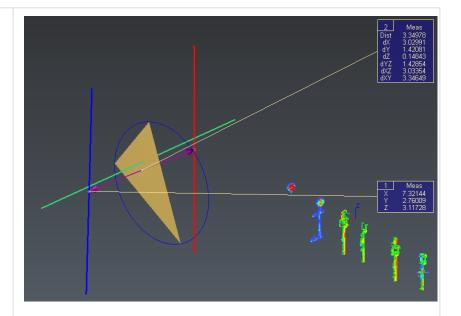
Launch the command <u>Distance</u> <u>Point Plane</u> and select the middle of the red line and the mesh.
