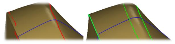
135 Polylines along curvature discontinuity; lines should be as on the right, they are smooth and correctly positioned on the discontinuities.
