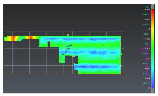
90 Check the levelness of a concrete floor
