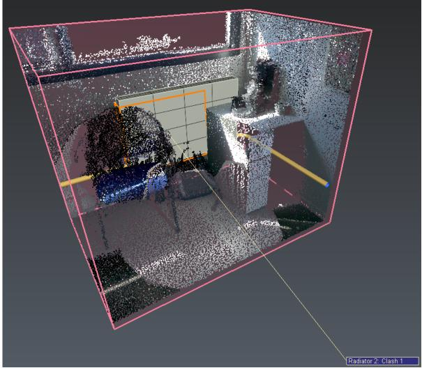
**79 Radiator 2: Clash 1**Heating pipe has 5 potential clashes with 677 points. Repeat the same process for each clash:
