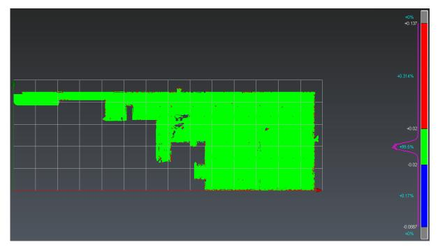
91 Check the flatness of a concrete floor
