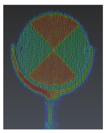
8 With the "Surveying target" option, you can click automatically and precisely the target center (with checkered pattern on the left, spherical on the right)
