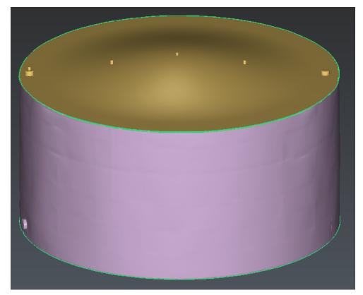
108 The tank is separated in 3 meshes: the shell, the top and the bottom
