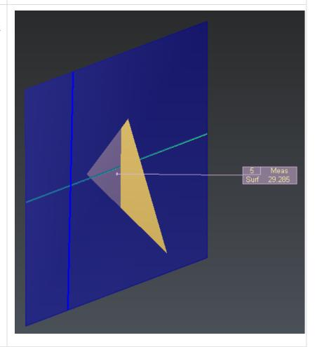
Launch the command Angle between Planes and select the plane and the mesh. Validate.
