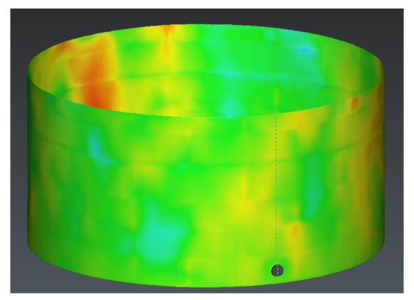
111 Parameters of the best cylinder are used to unroll the shell of the tank
