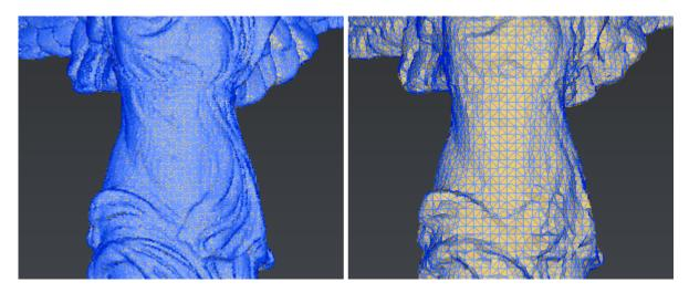
29 Regular Sampling: this method creates regular meshes where the size of the triangles depends on the average distance between points
