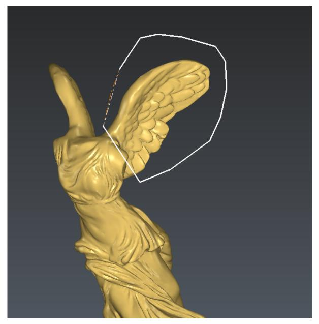
33 Cut a part of a mesh by selecting triangles inside a polygon
