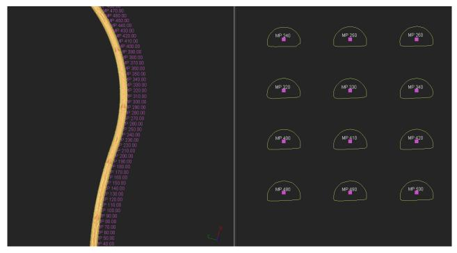
83 Create cross sections on a mesh along the neutral axis
