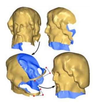
39 In the case of the file FillHoles.3dr, it is necessary to preserve continuity with the surface of the border to recreate the back of the head
