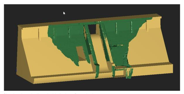
27 Cloud and mesh aligned with the best fit method
