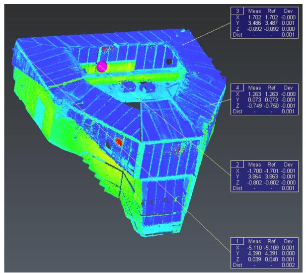
23 Labels to show deviations during the alignment according targets (less than 2mm in this case)
