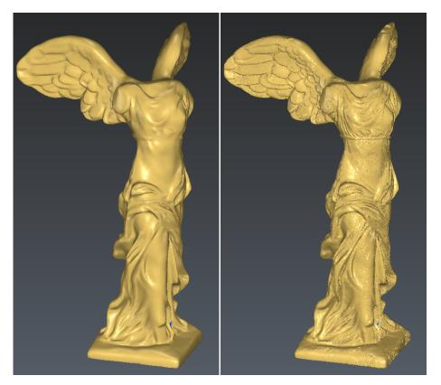
31 Comparison between the two refinement methods; Left: Interpolate new points: Right: Take points of the cloud
