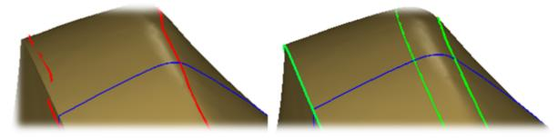
155 Polylines along curvature discontinuity; lines should be as on the right, they are smooth and correctly positioned on the discontinuities.
