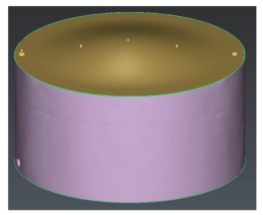
119 The tank is separated in 3 meshes: the shell, the top and the bottom
