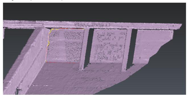
68 Planar contours extracted from a point cloud
