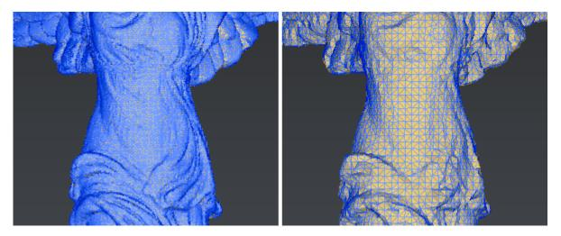
35 Regular Sampling: this method creates regular meshes where the size of the triangles depends on the average distance between points
