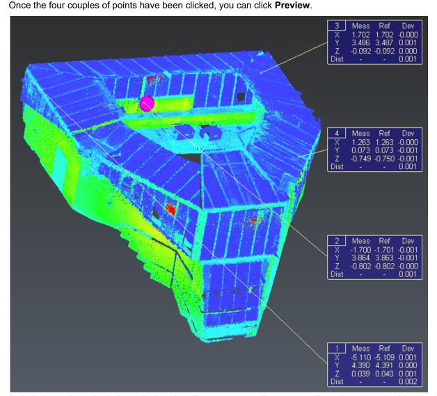
27 Labels to show deviations during the alignment according targets (less than 2mm in this case)
