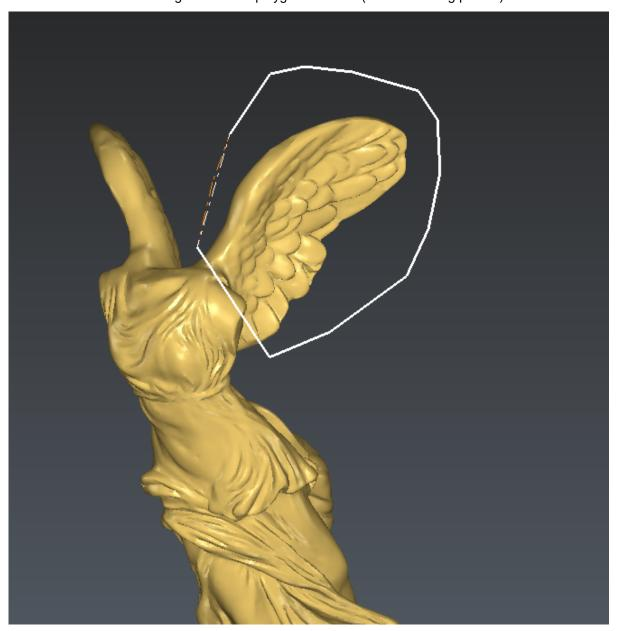
**39 Cut a part of a mesh by selecting triangles inside a polygon**Press **Enter** to validate the selection. Then do the same for the second wing.
