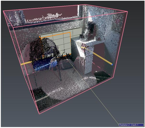
**88 Radiator 2: Clash 1**Heating pipe has 5 potential clashes with 677 points. Repeat the same process for each clash:
