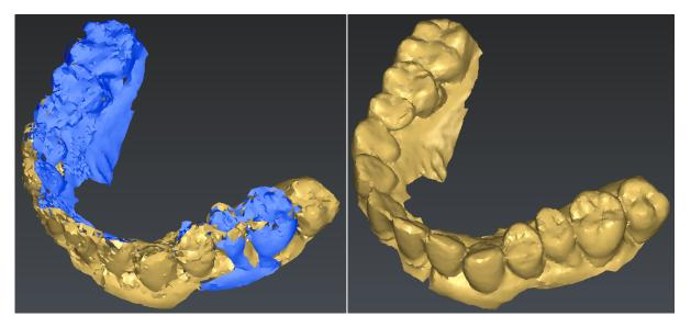
25 Comparison between two meshes with/without best fit alignment
