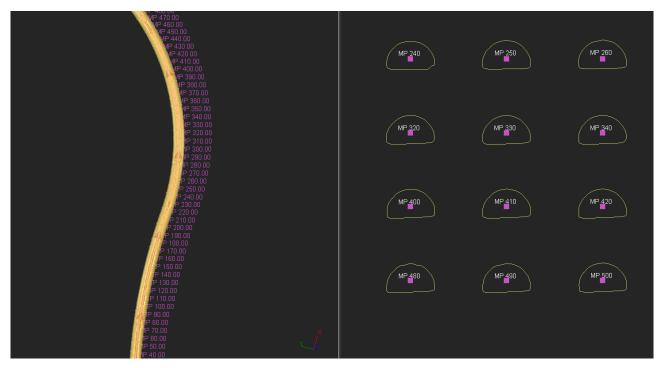
94 Create cross sections on a mesh along the neutral axis
