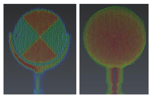
8 With the "Surveying target" option, you can click automatically and precisely the target center (with checkered pattern on the left, spherical on the right)
