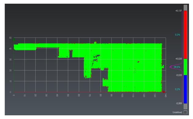
102 Check the flatness of a concrete floor
