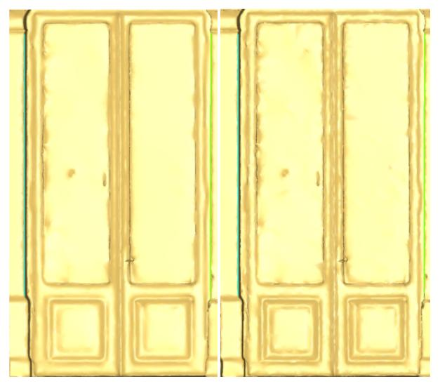
44 without deviation control (on the left); with deviation control (on the right)
