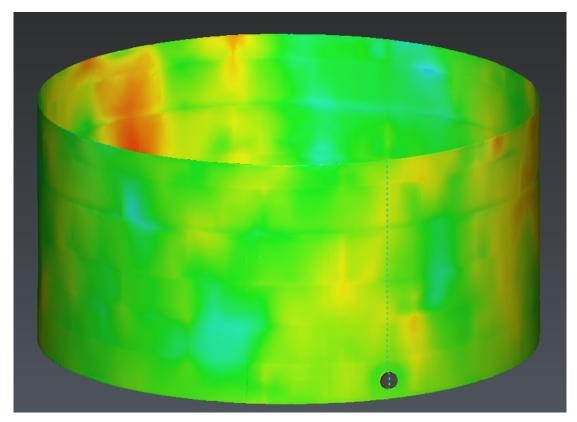
122 Parameters of the best cylinder are used to unroll the shell of the tank
