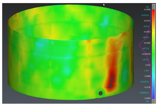
120 Compute the 3D deviations on the tank shell
