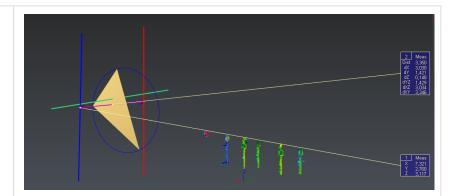
Launch the command Distance Point Plane and select the middle of the red line and the triangle.
