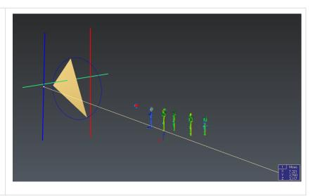
Launch the command Distance between Points and select the middle of the blue line and the middle of the red one.
