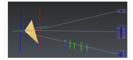
Launch the command Draw Plane and select the three vertices of the triangle. Validate the command.
