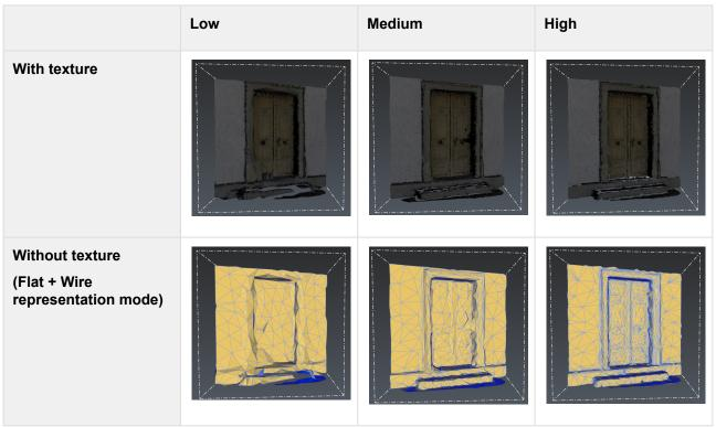
The evaluation mode is suitable to tune the mesh according to your needs and the computation time to spend.
