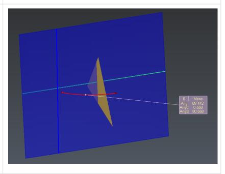
Now hide the plane and launch the command Angle between Lines and select the two visible lines.
