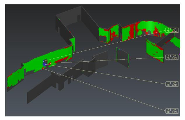
83 Inspected BIM and labels assigned to an issue Optionally, create another notes. Validate with **OK**.
