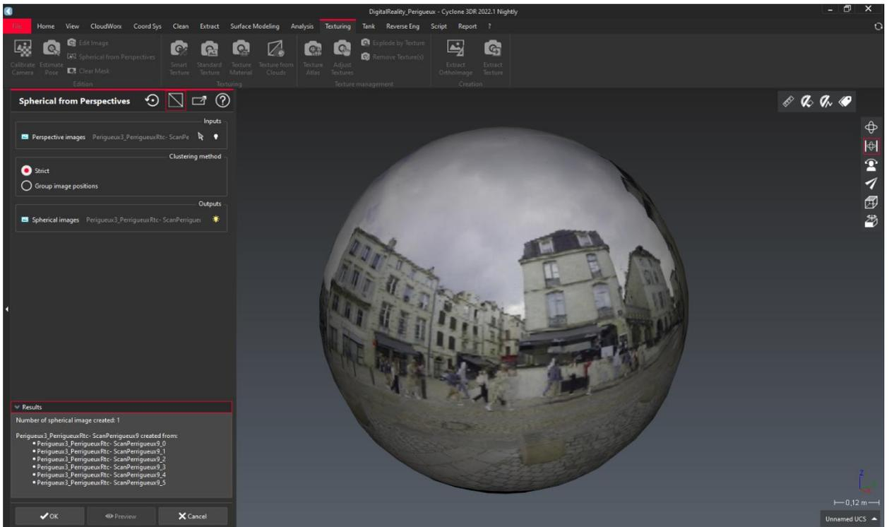
*Result from the grouping operation from the 6 cubic-face images to a single spherical image*
