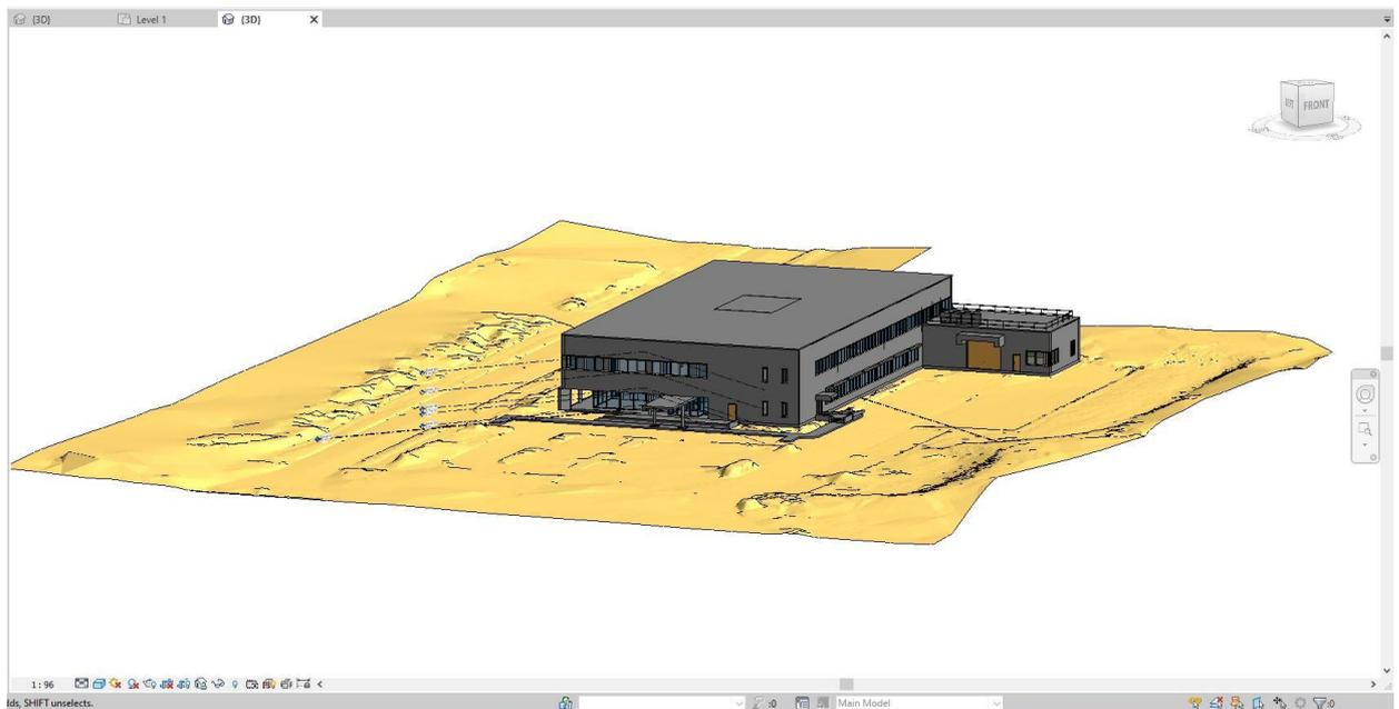
Note that any kind of mesh model in Cyclone 3DR can be exported to IFC with the new feature. That means that any refined models of an existing construction like a facade or a statue can be also exported to IFC, which can be helpful for Heritage applications. Consider with the 2022.1 release, that the IFC export classifies the exported objects to the IFCSite family only.
