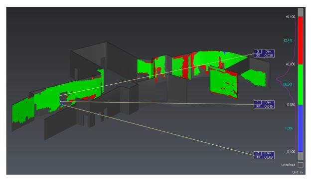
**81 Inspected BIM and labels assigned to an issue** Optionally, create another notes. Validate with **OK**.
