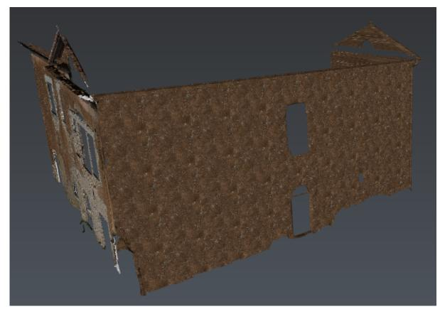
**148 Fig.3 Complete the texture with a repetitive pattern** Then remove, the repetitive texture on the last side using Adjust Textures.
