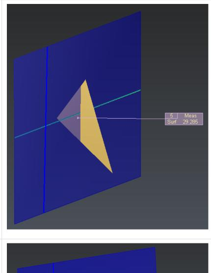
Launch the command Angle between Planes and select the plane and the mesh. Validate.
