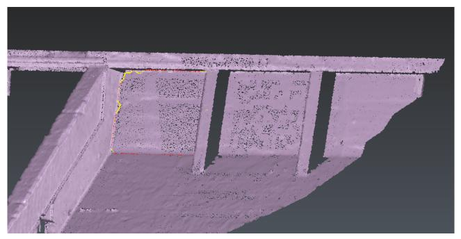
66 Planar contours extracted from a point cloud
