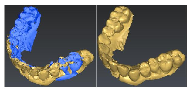
24 Comparison between two meshes with/without best fit alignment
