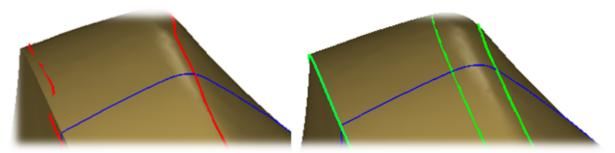
157 Polylines along curvature discontinuity; lines should be as on the right, they are smooth and correctly positioned on the discontinuities.
