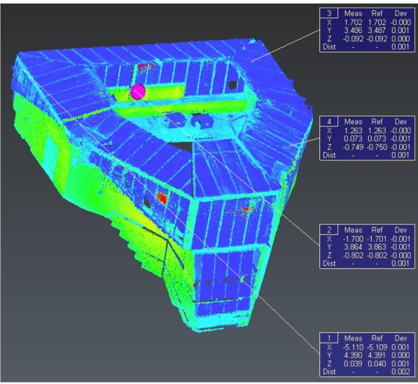
Unselect the option Apply Bestfit as we want to do an alignment according to targets only.
