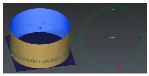
127 Display the section in 2D and in 3D on the tank
