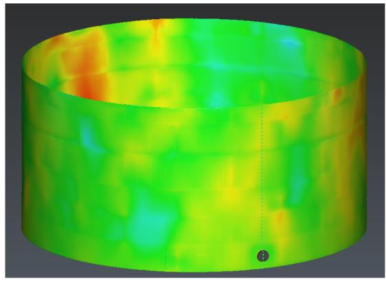
124 Parameters of the best cylinder are used to unroll the shell of the tank
