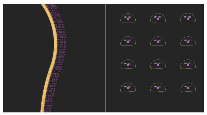
92 Create cross sections on a mesh along the neutral axis
