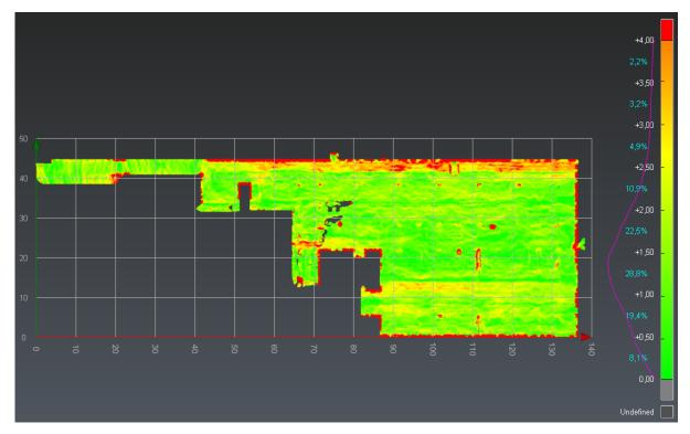
101 Check the slopes on a concrete floor
