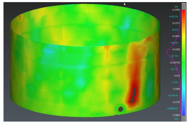
122 Compute the 3D deviations on the tank shell
