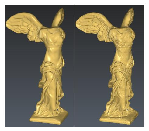
36 Comparison between the two refinement methods; Left: Interpolate new points: Right: Take points of the cloud
